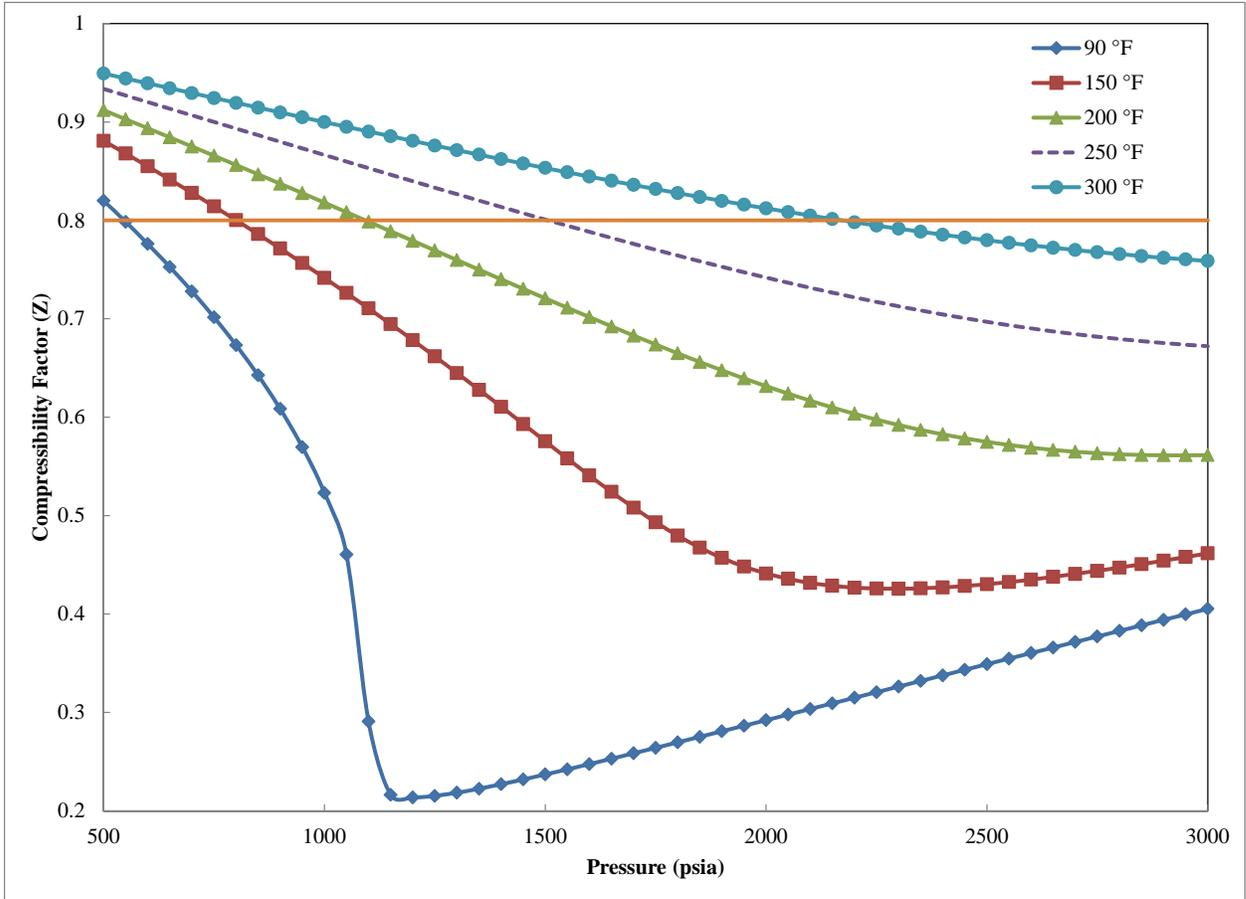
**Figure 1. Compressibility Factor of Pure CO<sub>2</sub> at Various Pressures and Temperatures.**
