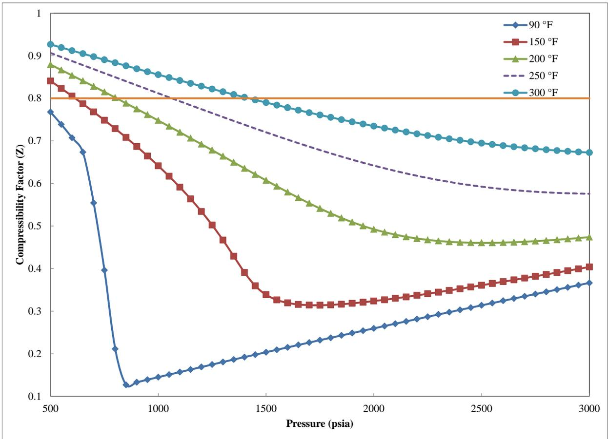
**Figure 2. Compressibility Factor of 50% CO<sub>2</sub> / 50% H<sub>2</sub>S (molar) Stream at Various Pressures and Temperatures.**
