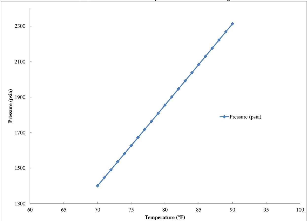
**Figure 5. Pressure of CO<sub>2</sub> at a Constant Volume as a Function of Temperature.**
