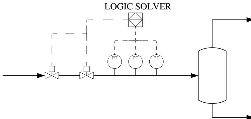
**Figure 6. Simple HIPPS for Overpressure Protection.**
