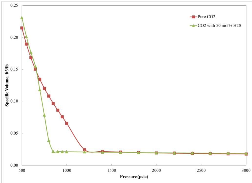
**Figure 3. Specific Volume of Pure CO<sub>2</sub> vs. CO<sub>2</sub> with 50 % H<sub>2</sub>S (molar) at 90 °F.**
