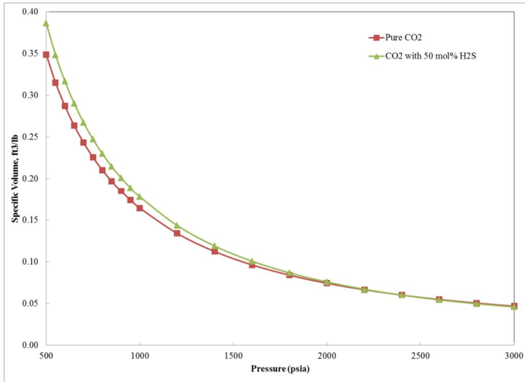
**Figure 4. Specific Volume of Pure CO<sub>2</sub> vs. CO<sub>2</sub> with 50% H<sub>2</sub>S (molar) at 300°F.**
