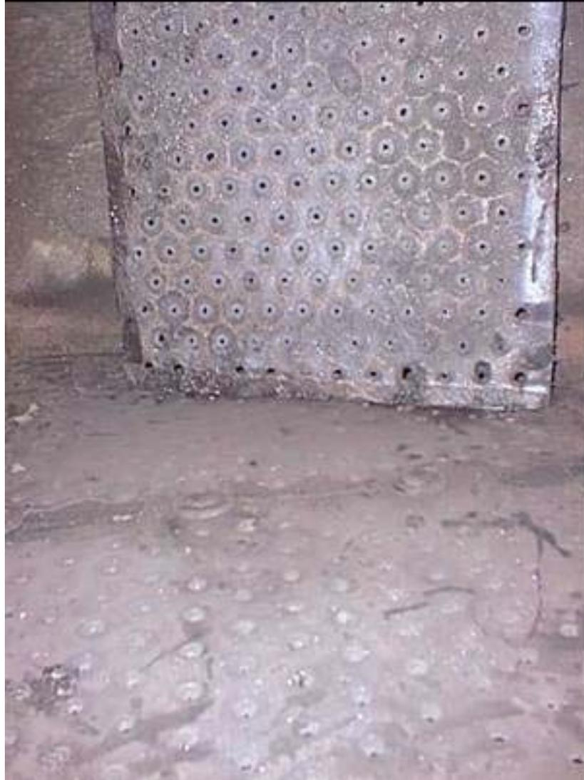
**Figure 3. Fouling of Sieve Tray in Sour Water Stripper Service [12].**
