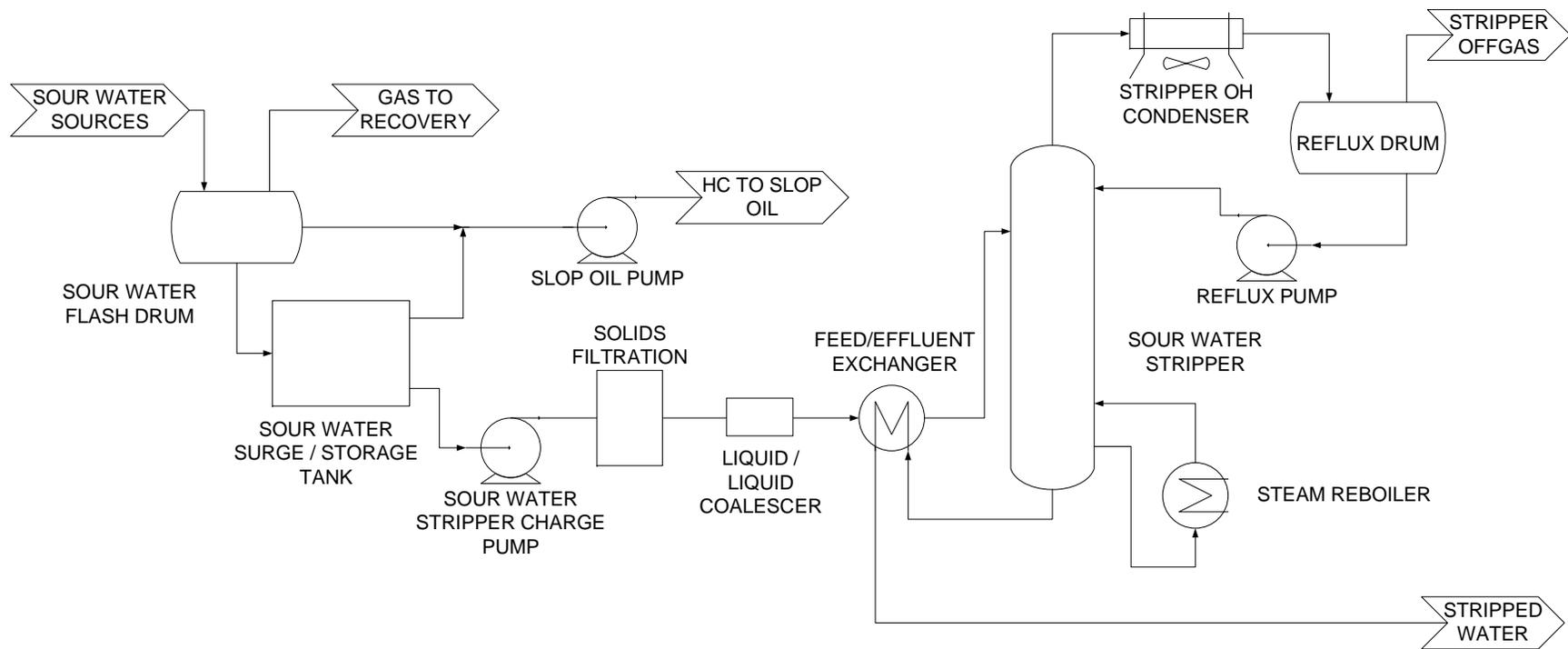
**Figure 1. Simplified Process Flow Diagram for Sour Water Stripper.**
