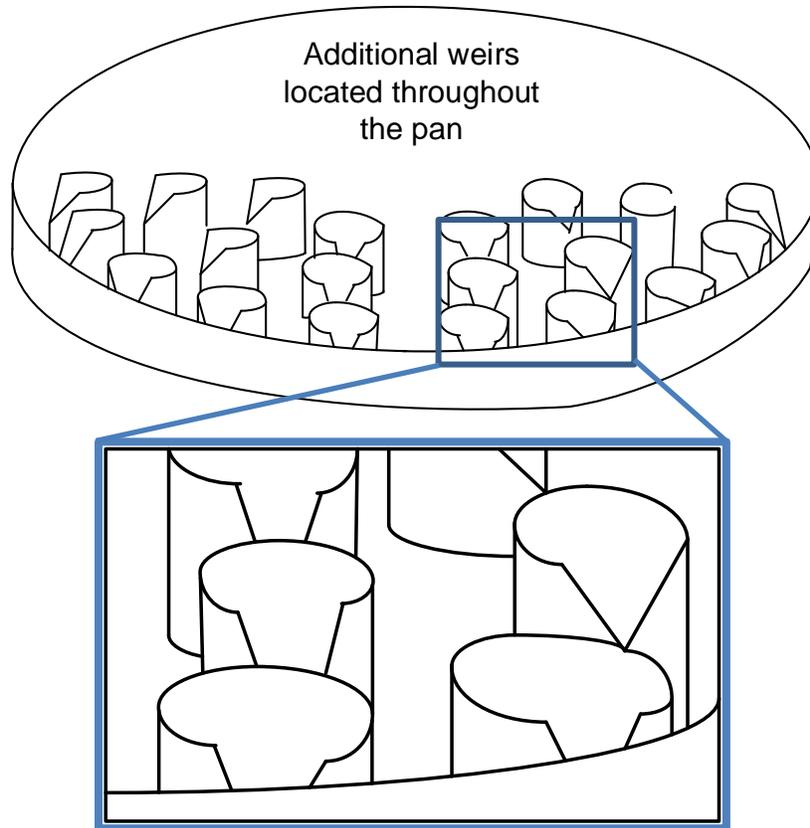
**Figure 6. Example Weir Riser Pan Distributor**
