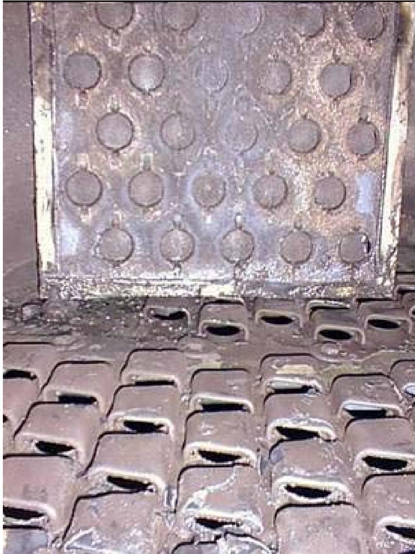
**Figure 4. Example of Tray Fouling in Sour Water Stripper Service [12].**
