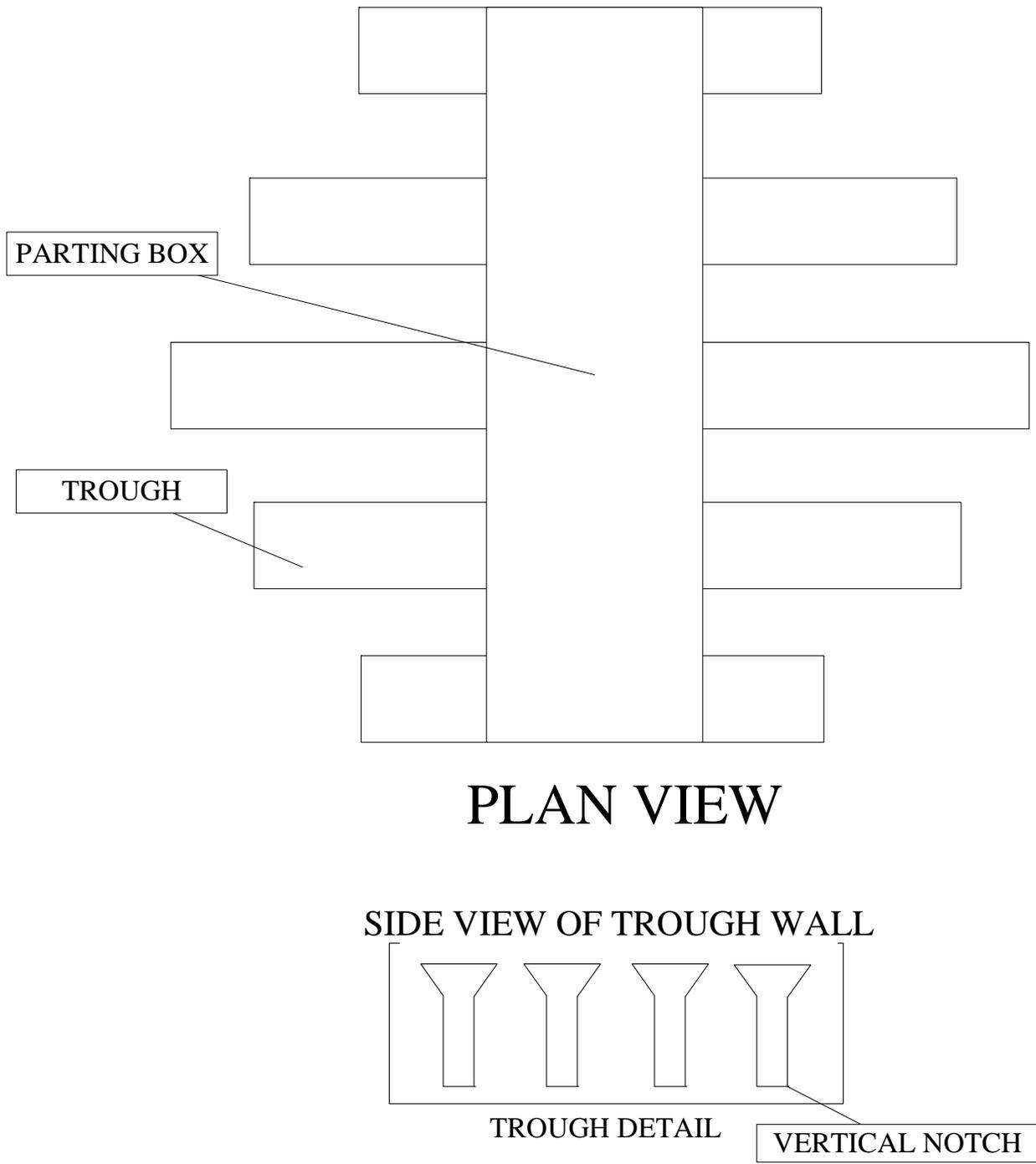
**Figure 7. Sketch of Trough Style Distributor**
