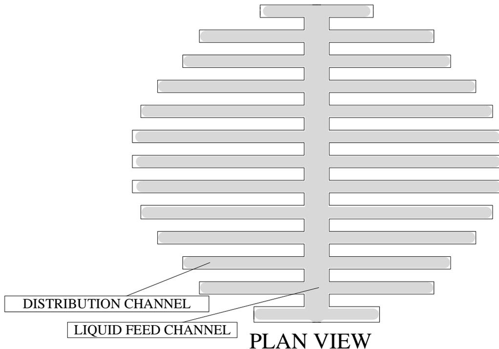
HOLE SIZE AND DENSITY SHOULD BE OPTIMIZED TO THE EXTENT ALLOWED BY THE OPERATING CONDITIONS OF THE DISTRIBUTOR.
