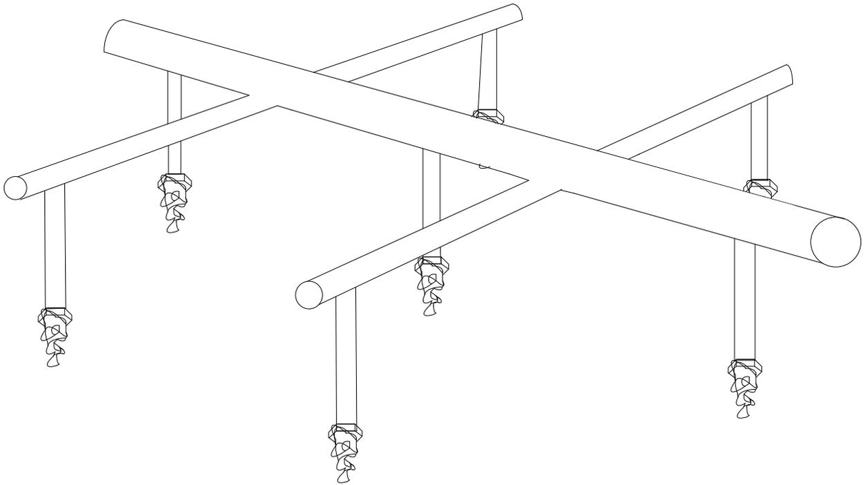
**Figure 8. Example Spray Header Liquid Distributor**
