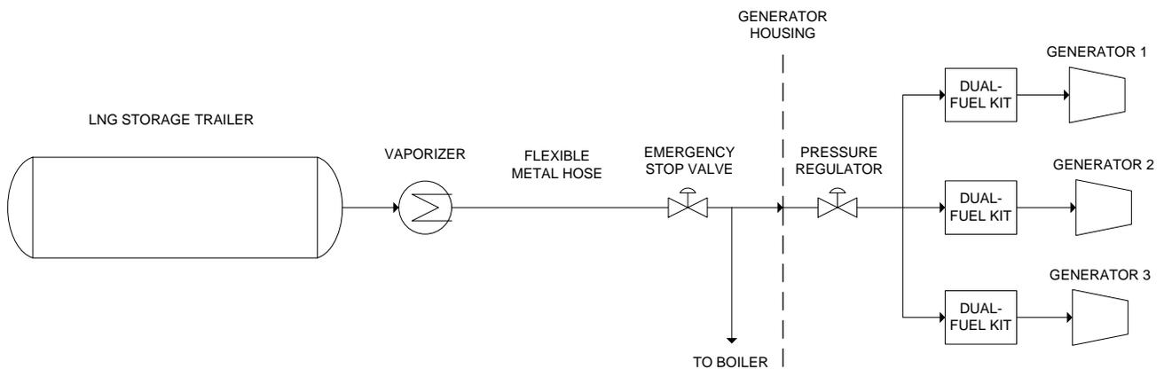
**Figure 1 Overview Schematic of LNG System**
