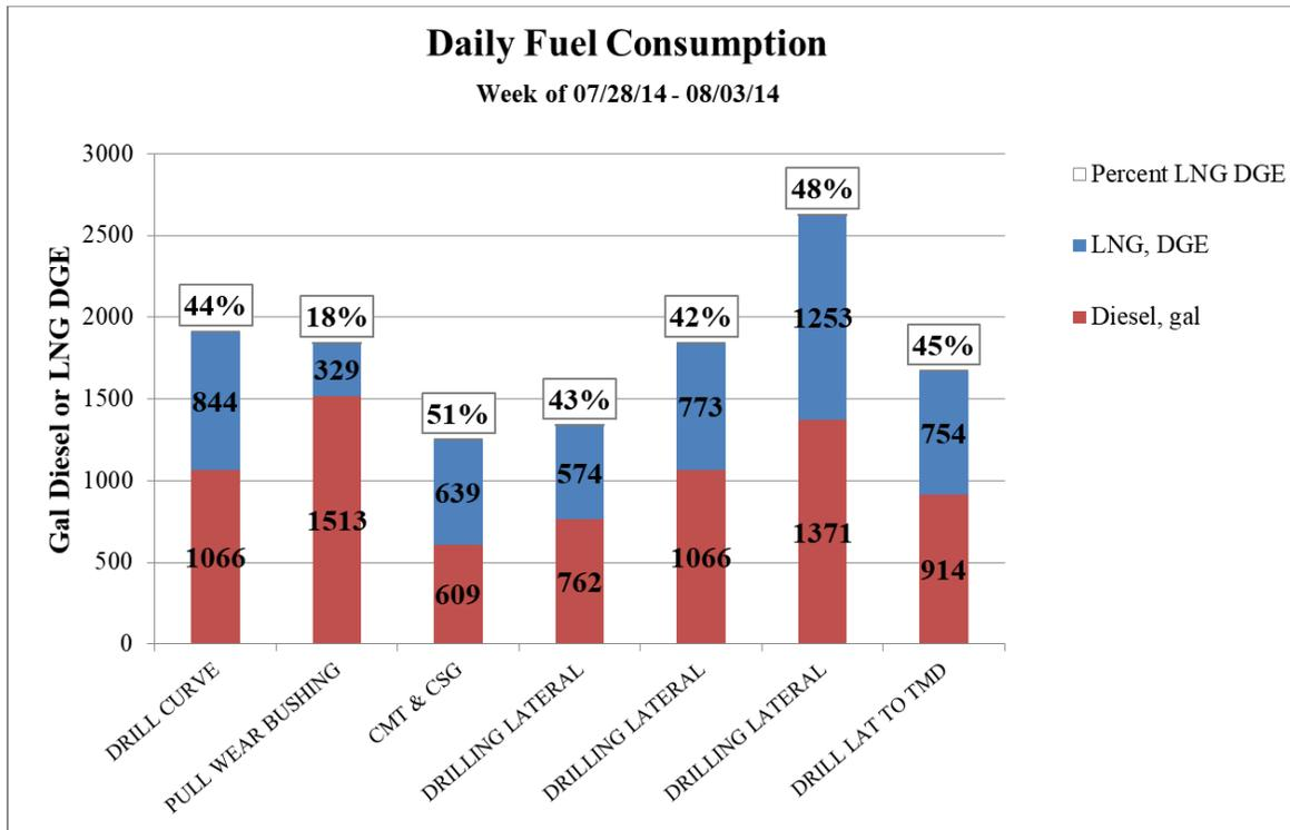
**Figure 6 Example Weekly Drilling Report Graph: Daily Fuel Consumption**
