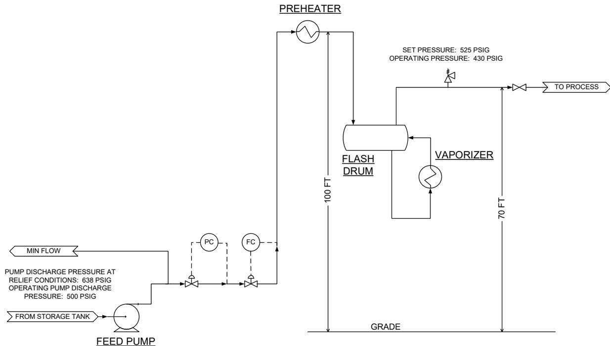
**Figure 3. Simplified Process Diagram for Closed Outlets Scenario.**
