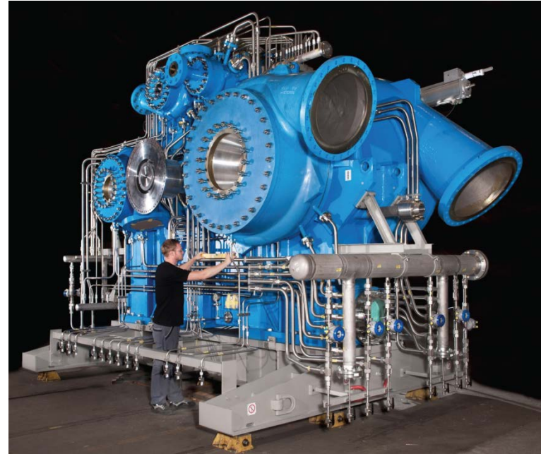
8-Stage, 15 MW Wet CO 2 Compressor Image courtesy of MAN Energy Solutions
