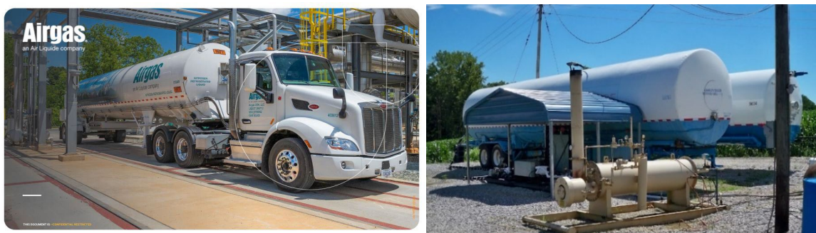
Fig. 5. (a) transport truck for refrigerated liquid, figure courtesy of Airgas an Air Liquide Company; (b) portable liquid CO 2 storage containers.
