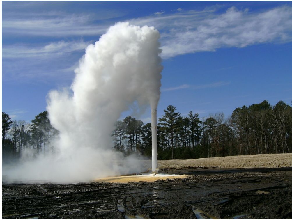
Figure 1. Example of Dry Ice Formation Due to Venting Liquid CO 2 .
