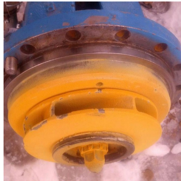
Sulfur-containing Solid on liquid CO 2 pump impeller in Distillation Plant.
